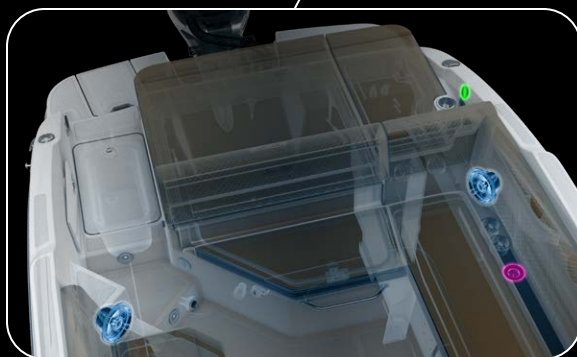
ARX remote unit and Apollo™ Series speakers
